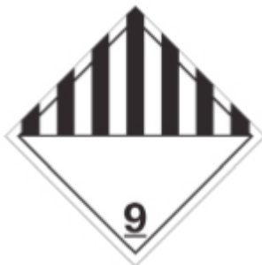
Figure 3. Identification label UN3480 Class 9
